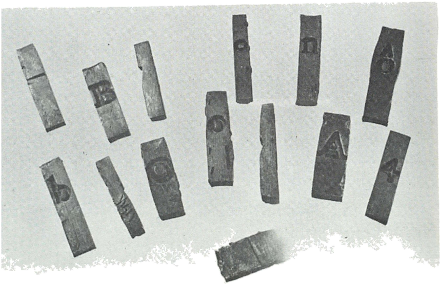
FIG. 6. Sixteenth-century matrices for the Canon Roman of François Guyot. The one in the top right-hand corner of the photograph has not been justified. Museum Plantin-Moretus (MA 131b).
