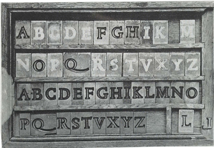
FIG. 8. Matrices for 5-line Pica Roman capitals of the 16th century belonging to Joh. Enschedé en Zonen of Haarlem. Lead matrices in the top two rows are believed to have been struck with the brass letters, some of which are shown fitted into them. One of the brass letters is lying on the bottom right-hand corner of the box.
