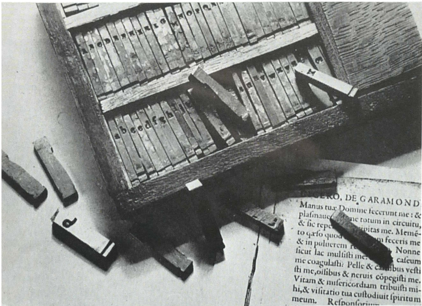
FIG. 4. Matrices for the Pica Roman face bought by Bishop Fell in 1672. Photograph by J. W. Thomas.
