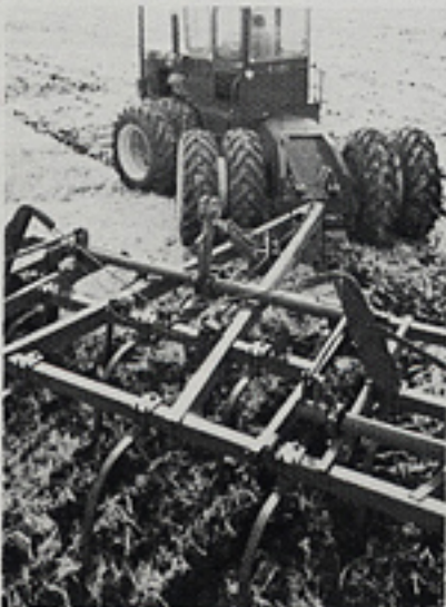
This unique four-wheel drive farm tractor powered by a Cummins compact V diesel tills the soil.
